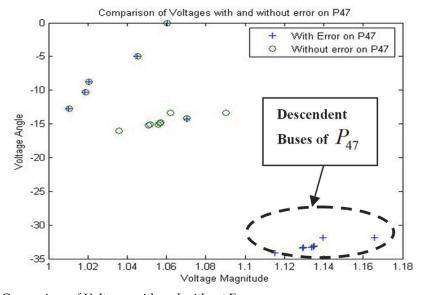
Fig. 3. Comparison of Voltages with and without Errors
