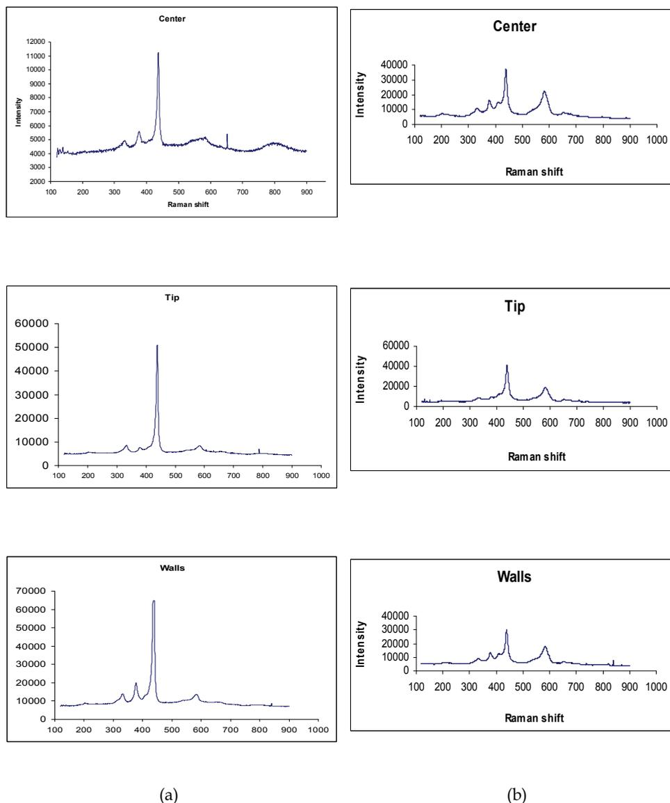
Fig. 2. (a) and (b) are plots of micro-Raman spectra of ZnO and Li: ZnO at different position. To study the quality of the crystal the strongest Raman active peak at 437cm<sup>-1</sup> was intensity normalized and a Gaussian fit was applied to get the area and width under each curve for different regions given in fig. 3(a) and 3(b).
