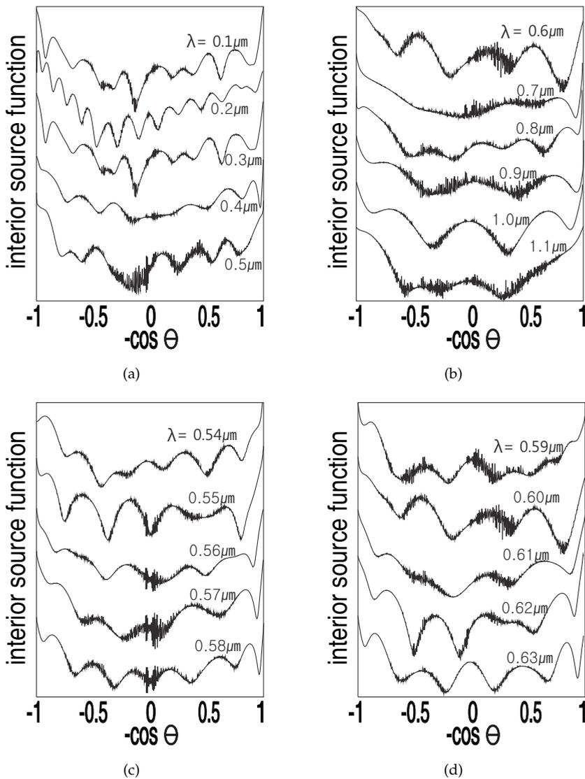
Fig. 6. Source functions vs.  $\cos(\text{angle})$  for a single-layer microsphere of 500 nm radius, the crystal size of 2.17 nm, and many different wavelengths. (a) For the wavelengths from 100 nm to 500 nm. (b) For the wavelengths from 600 nm to 1100 nm. (c) and (d) More detailed data for wavelengths between 540 nm and 630 nm. The number of surface peripheral elements were 725. The refractive index on the unit cell edge was chosen to be  $3.23+i0.01$ .
