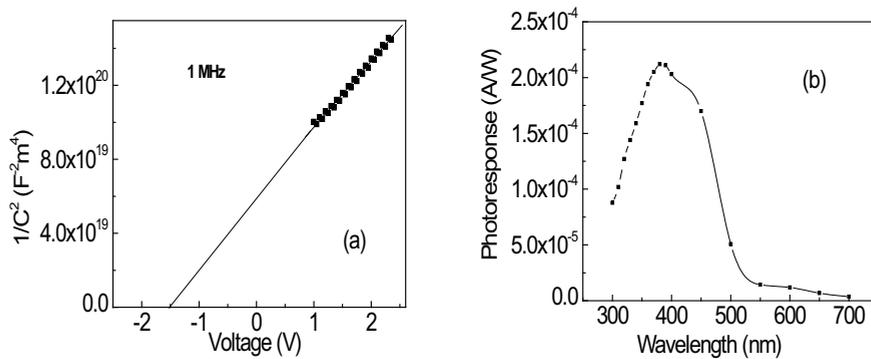
Fig. 6. Dependence of  $1/C^2$  value on applied voltage (a) and spectral photoresponse (b) of ZnSe/p-Si Schottky diode. [Reprinted with permission from (Venkatachalam et al., 2006). Copyright @ IOP Publishing Ltd (2006)].
