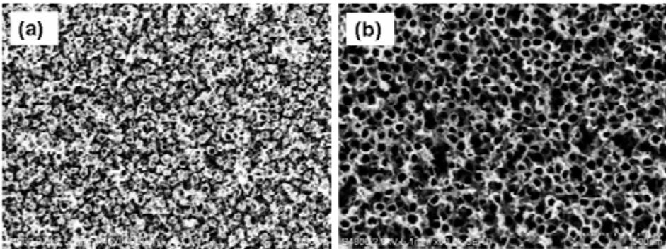
Fig. 14. SEM images of Ti/ITO/glass and Ti/Si after anodization in glycerol containing 2.5 vol. % H<sub>2</sub>O + 0.5wt. % NH<sub>4</sub>F at 30 V and ethylene glycol containing 2.0 vol. % H<sub>2</sub>O + 0.3wt. % NH<sub>4</sub>F at 20 V for 240 min (a) and 180 min (b), respectively.
