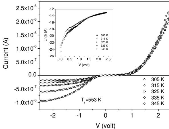
Fig. 4. Forward and reverse current versus voltage characteristics of ZnSe/Au Schottky diode. The inset of Fig.4 shows the plot of voltage versus  $\text{Ln}I$ . [Reprinted with permission from (Venkatachalam et al., 2006). Copyright @ IOP Publishing Ltd (2006)].
