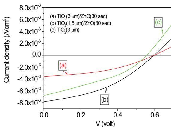
Fig. 17. Photocurrent density-voltage characteristics of dye-sensitized solar cell based on TiO<sub>2</sub> and ZnO/TiO<sub>2</sub> films.
