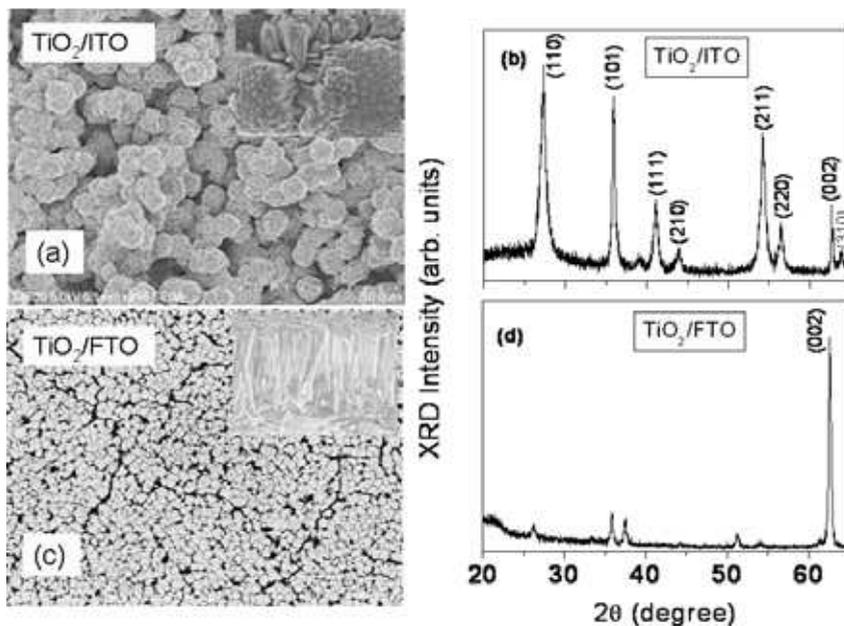
Fig. 9. Scanning electron microscope images and X-ray diffraction patterns of titanium dioxide films on different substrates; (a and b) TiO<sub>2</sub> film on ITO/glass, (c and d) TiO<sub>2</sub> film on FTO/glass.
