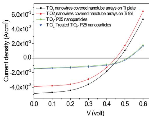
Fig. 13. Photocurrent density-voltage characteristics of dye-sensitized solar cells based on TiO<sub>2</sub> nanotube arrays and nanoparticles.
