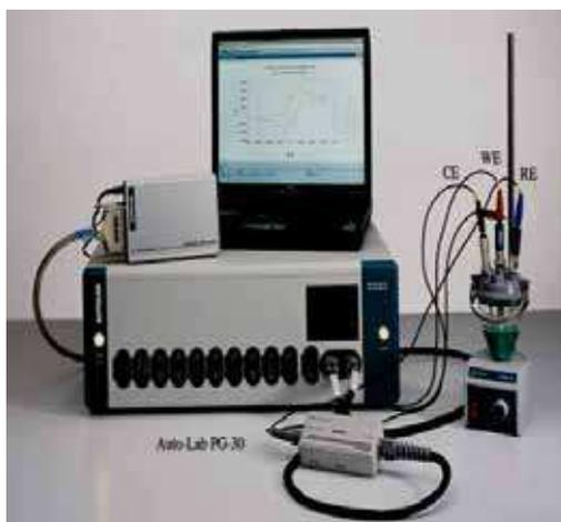
Fig. 1. Electrochemical etching setup for fabricating PS layers
