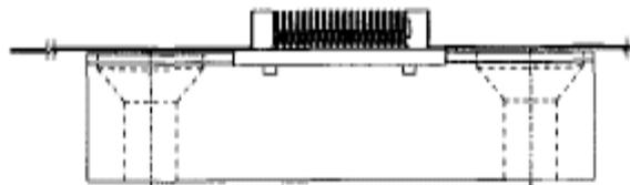
Fig. 16. 20 bar, 0.8 cm<sup>2</sup> array (1500 W/cm<sup>2</sup>) mounted on a copper block. This design minimizes overall packaging costs.
