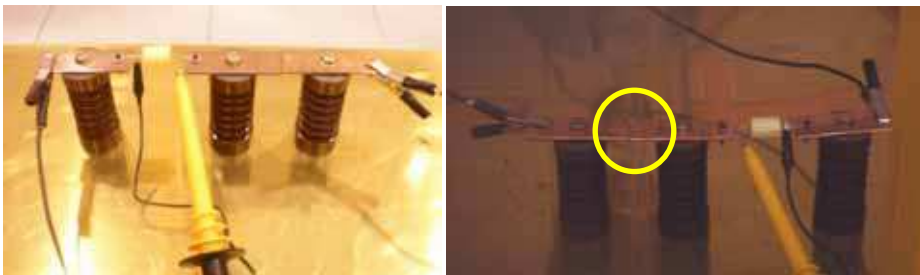
Fig. 18. Flashover occurred between the gap (spark in the yellow circle)
