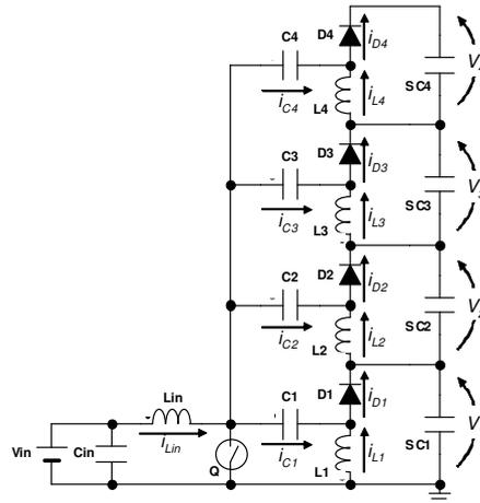
Fig. 3. Single-switch cell/module voltage equalizer using multi-stacked SEPICs.
