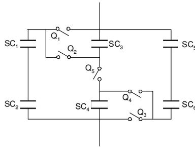
Fig. 14. Reconfigurable series-parallel SC energy storage unit.
