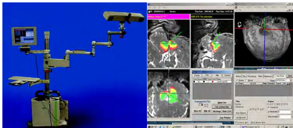
Fig. 5. Intraoperative neuronavigation system (PRS navigator; Toshiba Medical Co. Ltd., Tokyo, Japan) used in intelligent operating theater of TWUM ( left ) and its screen with color-coded safety areas of the tumor resection ( right ), showing areas located less than 5 mm, between 5 and 10 mm, and more than 10 mm to the pyramidal tract, which are demarcated, respectively, as red, yellow, and green.
