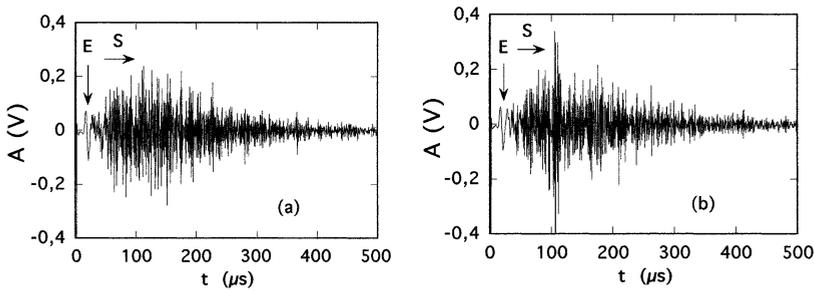
Fig. 4. Transmitted ultrasonic signal through a dry glass beads packing with  $d = 0.4 - 0.8$  mm, detected by a transducer of diameter 2 mm and external normal stress  $P = 0.75$  MPa: (a) First loading; (b) reloading. (Reprinted from Jia et al., Phys. Rev. Lett. 82, 1863 (1999))
