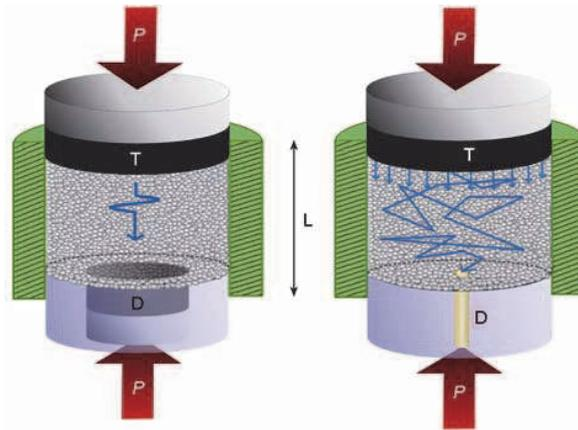
Fig. 1. Multiple scattering of elastic waves in a confined granular packing under stress  $P$ . “ $T$ ” and “ $D$ ” correspond to a large source transducer and a small detector, respectively. (Reprinted from Jia et al., Chinese Sci. Bull. 54, 4327 (2009))
