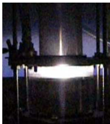
Fig. 27. Schematic (left) of the PLS reactor with the DC discharge in a reverse vortex gas flow of Tornado type with a "liquid" electrode and photo (right) of the TORNADO-LE working in ethanol-water solution.
