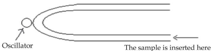
Fig. 7. U-shaped tube of digital density meter.
