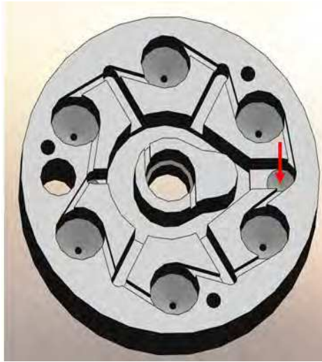
Fig. 13. Plate of fuel. Red arrow - inlet of fluid.
