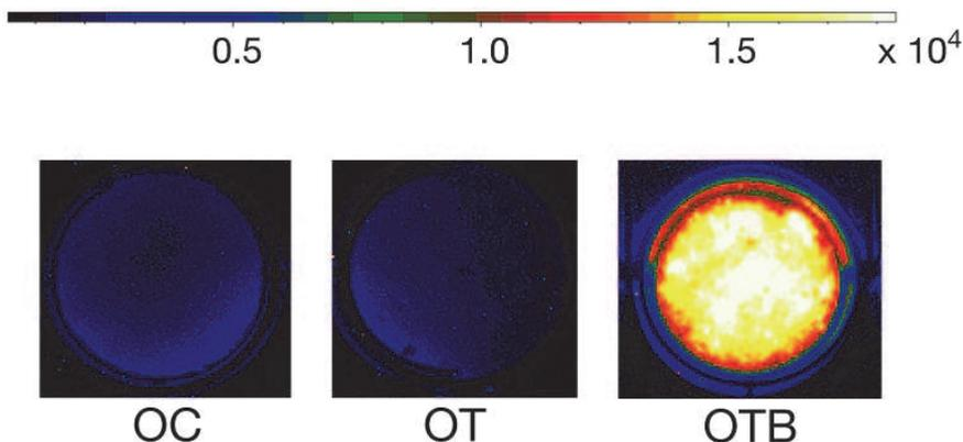
Detection image of photon emission from OC, OT and OTB using a charge-coupled device camera. OC, lyophilized okara; OT, lyophilized okara fermented by *R. oligosporus*; OTB, lyophilized OT-banana combination. The lyophilized sample (30 mg), saturated  $\text{KH}_2\text{CO}_3$  in 10% (Vol/Vol) acetaldehyde (1000  $\mu\text{L}$ ), and 0.6%  $\text{H}_2\text{O}_2$  (1000  $\mu\text{L}$ ) were mixed in a 24-well micro titer plate.
