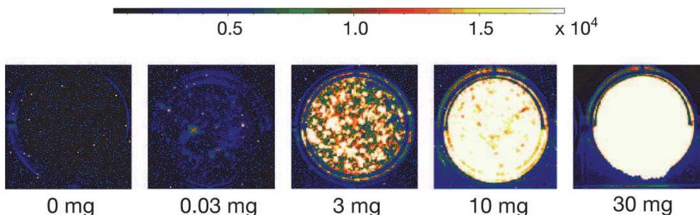
Imaging detection of photon emission from OTB 4:3 using a charge-coupled device camera. The lyophilized OTB 4:3 (0 mg, 0.03 mg, 3 mg, 10 mg, and 30 mg), saturated  $\text{KH}_2\text{CO}_3$  in 10% (Vol/Vol) acetaldehyde (1000  $\mu\text{L}$ ), and 0.6%  $\text{H}_2\text{O}_2$  (1000  $\mu\text{L}$ ) were mixed in a 24-well micro titer plate.
