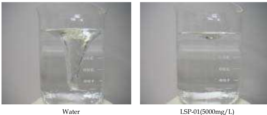
Fig. 4. Photos of water and a drag-reducing solution stirred in a beaker
