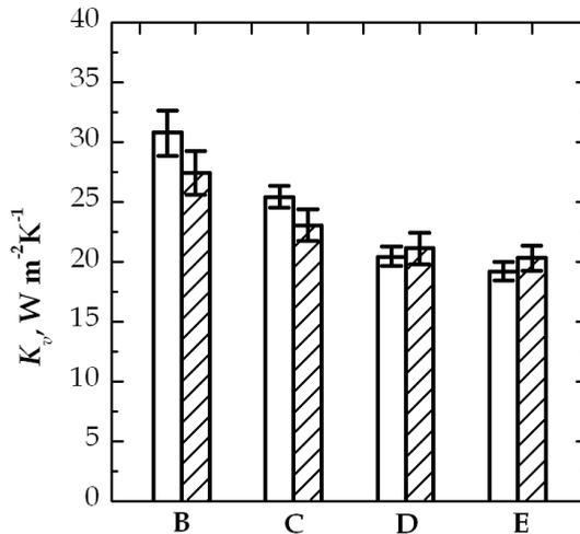
Fig. 10. Heat transfer coefficient (at  $P_c=10$  Pa) of the four groups of vials ( $V_2$  type, silane treated) in case of two different loading configurations: (void bars) the lot of vials is loaded on the heating shelf; (filled bar) the lot of vials is loaded on the heating shelf and enclosed by an external metal band
