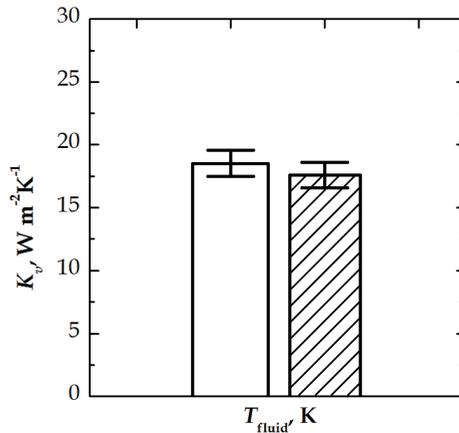
Fig. 5. Effect of  $T_{\text{fluid}}$ , and in turn of chamber gas temperature, on the value of  $K_v$  for the vial  $V_2$  processed in the laboratory freeze-dryer. Both measurements were carried out at  $P_c=10$  Pa, while the fluid temperature was set to: (□)  $T_{\text{fluid}}=275$  K; (▨)  $T_{\text{fluid}}=253$  K
