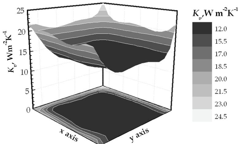
Fig. 4. Contour plot of the heat transfer coefficient for vials  $V_1$  (loaded directly over the heating shelf) as measured over a lot. The primary drying phase was run at  $T_{\text{fluid}}=263$  K and  $P_c=5$  Pa. Results refer to a half of the batch
