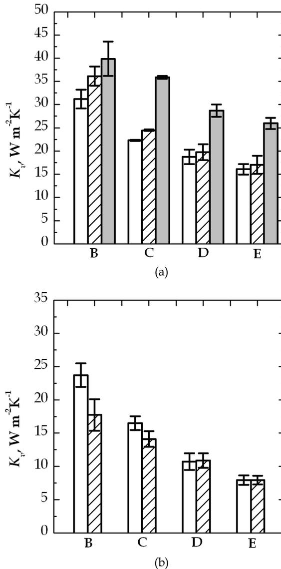
Fig. 12. Comparison between experimental values of  $K_v$  for the various groups of vials ( $V_4$  type). (a) Influence of various loading configurations: vials loaded on a stainless steel tray (□), a polystyrene tray (▨) and directly on the heating shelf (■); (b) values measured in two pieces of equipment of different size: (□) laboratory and (▨) industrial scale dryer
