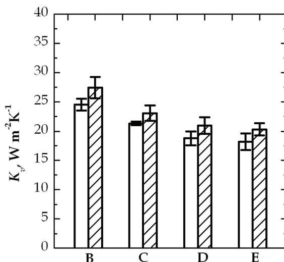
Fig. 9. Heat transfer coefficient of the four groups of vials ( $V_2$  type) in case they underwent a silane coating treatment (void bars) or not (filled bar). The lot of vials is loaded on the heating shelf and enclosed by an external metal band. The measurement was carried out at  $P_c=10$  Pa
