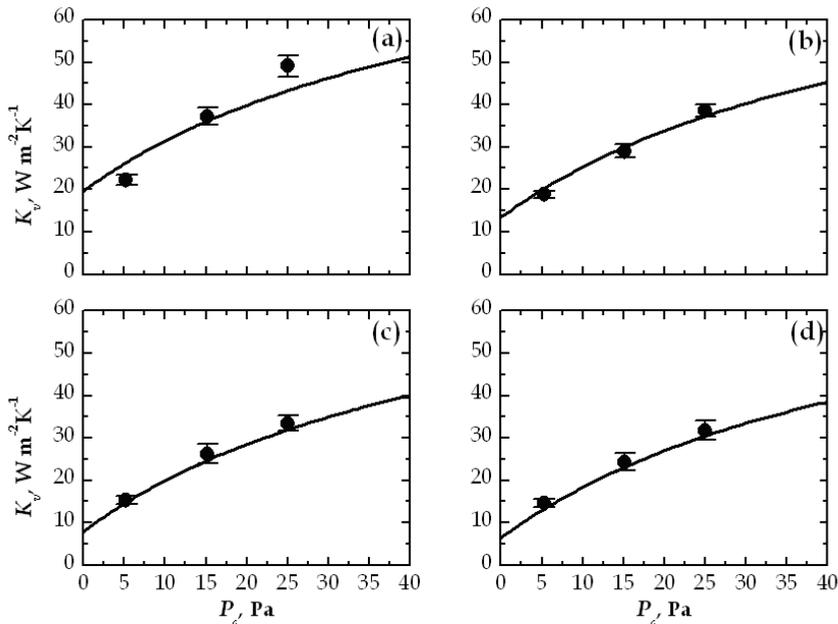
Fig. 6. Values of  $K_v$  vs.  $P_c$  for the four groups of vials (type  $V_1$ ) identified in Table 1: (a) vials B; (b) vials C; (c) vials D and (d) E
