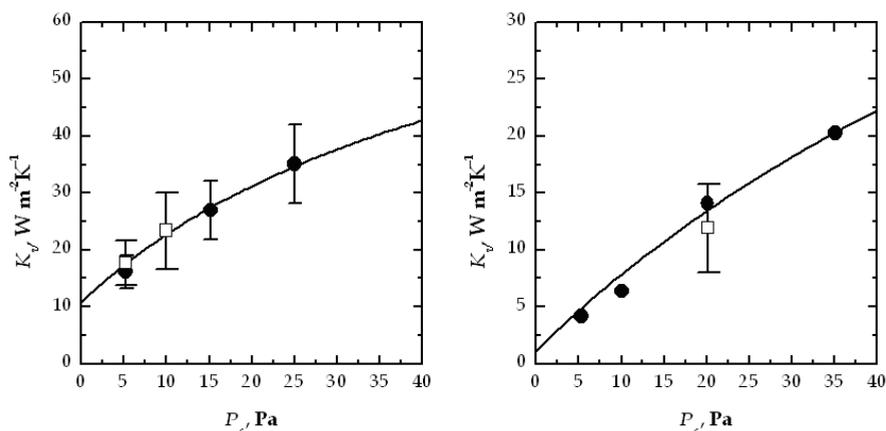
Fig. 3. Effect of chamber pressure on the value of  $K_v$  for the vial V<sub>1</sub> (left-side graph) and a stainless steel tray (right-side graph) processed in the laboratory freeze-dryer. The values calculated using the theoretical model, and the parameters of Table 3, are also displayed (solid line) together with the value estimated by pressure rise test technique ( $\square$ )
