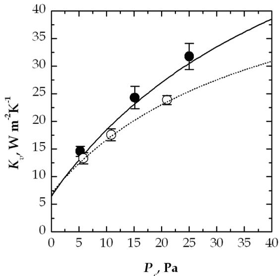
Fig. 8. Comparison between the value of  $K_v$  vs.  $P_c$  for vials subset E (processed in the laboratory freeze-dryer) in case of two different container geometries: (●)  $V_1$  and (○)  $V_2$  type. The values calculated using the theoretical model are also displayed: (solid line) vials  $V_1$  and (dotted line)  $V_2$
