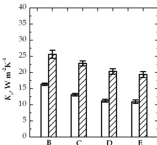
Fig. 11. Heat transfer coefficient (at  $P_c=10$  Pa) of the four groups of vials ( $V_3$  type) in case of two different loading configurations: (void bars) the lot of vials is loaded on a metal tray; (filled bar) the lot of vials is loaded on the heating shelf and enclosed by an external metal band
