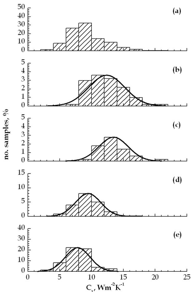
Fig. 7. Distribution of  $C_1$  of vials  $V_1$  for: (a) the entire lot; (b) vials B; (c) vials C; (d) vials D and (e) vials E. The solid line is the Gaussian distribution calculated according to the mean value and standard deviation reported in Table 3
