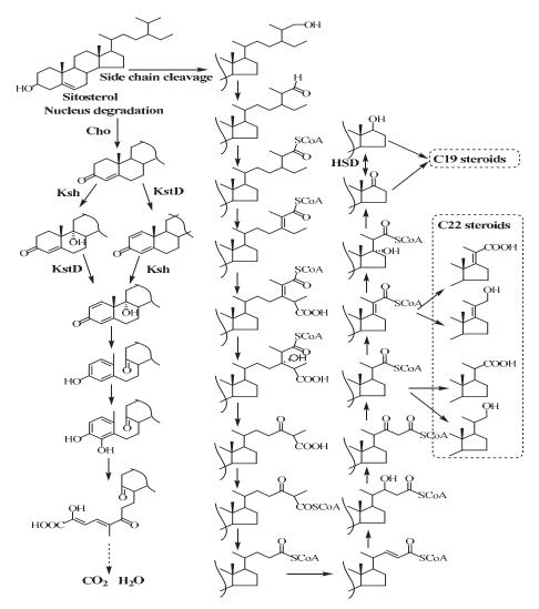
Fig. 4. Catabolic pathway of phytosterols (with  $\beta$ -sitosterol as substrate). (HSD represents the enzyme 17 $\beta$ -hydroxy steroid dehydrogenase.) (Kieslich, 1985; Szentirmai, 1990; van der Geize, *et al.*, 2007)
