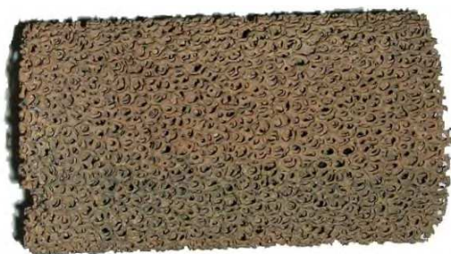
Fig. 8. Structured steam reforming catalyst
