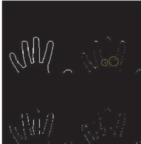
Fig. 17. A mistake in horizontal information detection in wavelet domain due to bad hand positioning.
