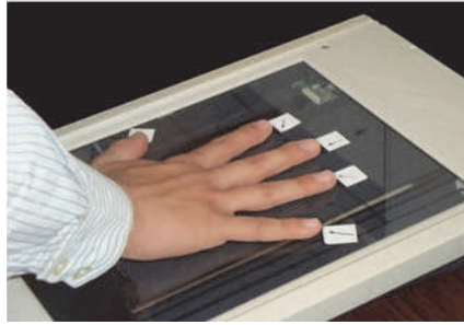
Fig. 4. Pegs on the scanner for hand positioning.
