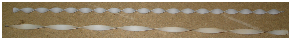
Fig. 6. Tapes with a minimum ( S/d = 2.5 ) and maximum ( S/d = 6 ) relative pitches of twisting
