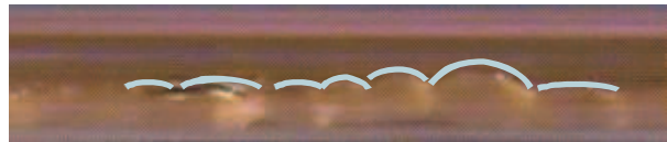
Fig. 9.2a. Liquid behaviour of the butanol aqueous solution (7.15 wt%) (Run 1a).
