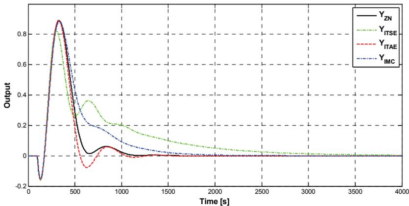
Fig. 12. Results of tuning for the model obtained in the remote station. The step response of the load variation of original tuning ZN ( $Y_{ZN}$ ) and some common methods based on model ( $Y_{ITSE}$ ,  $Y_{ITAE}$  and  $Y_{IMC}$ ).
