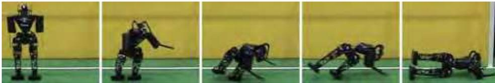
Figure 10. Diving motion of the goalkeeper
