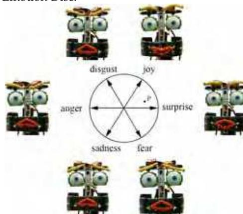
Figure 7. The two-dimensional space in which we compute the robot's emotional state. The images show the six basic facial expressions
