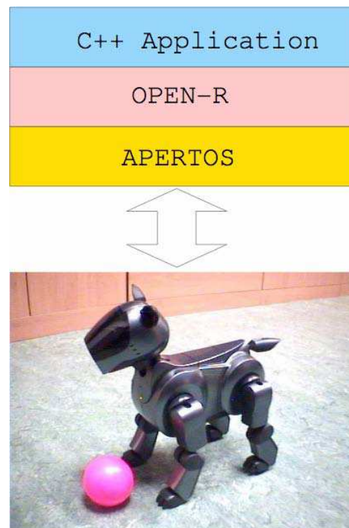
Figure 5. Software architecture for programming Sony Aibo robot
