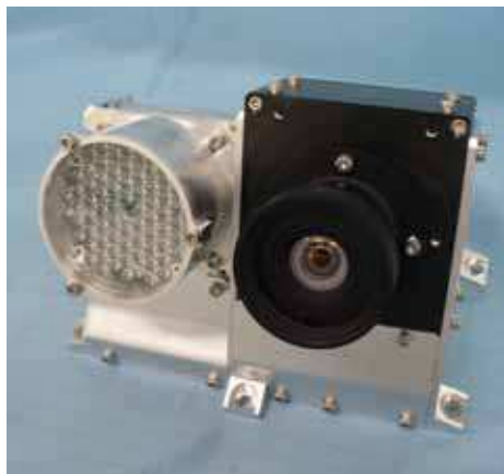
Fig. 4. Monitoring camera mounted on GOSAT © Meisei Electric Co., Ltd.
