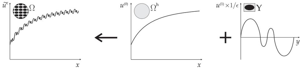
Fig. 2. Illustration of the asymptotic expansion homogenisation first-order approximation for the displacement field for a one-dimensional case. The displacement field in  $\Omega$  is approximated adding the  $Y$ -periodic microscale first-order fluctuations to the homogenised macroscale  $\Omega^h$  field.
