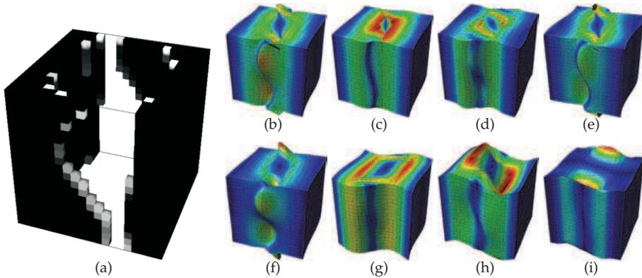
Fig. 10. Multiobjective topology optimisation, using the local approach, for a 3-D RUC ( $w^t=0.5$ ): (a) material distribution, (b) thermal expansion ( $\Psi$ ), (c) conductivity ( $\Upsilon$ ) and (d-i)  $\chi_{11}$ ,  $\chi_{22}$ ,  $\chi_{33}$ ,  $\chi_{12}$ ,  $\chi_{23}$  and  $\chi_{13}$  characteristic displacement modes.
