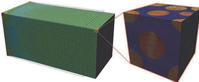
Fig. 6. Equivalent von Mises stress on the microscale, obtained with the localisation procedure on a Gauss point of a macroscale finite element (Oliveira et al., 2009).
