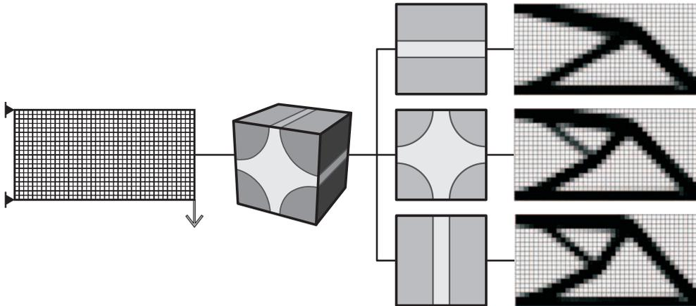
Fig. 7. Topology optimisation results using different reinforcement orientations.
