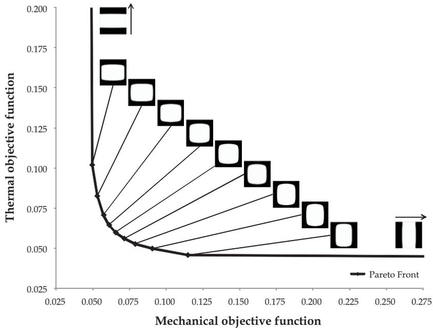
Fig. 8. Square RUC microscale optimisation results: Pareto front for a 2-D mechanical/thermal multiobjective problem.
