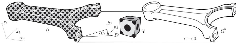
Fig. 1. Heterogeneous thermoelastic material  $\Omega$  and representative unit-cell  $Y$  used in the microscale problem of the asymptotic expansion homogenisation, resulting, with  $\epsilon \rightarrow 0$ , on the homogeneous material  $\Omega^h$ .
