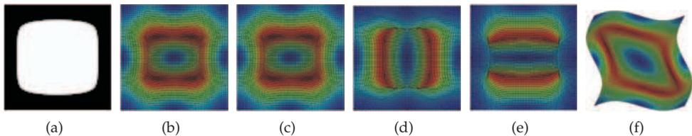
Fig. 9. Multiobjective topology optimisation, using the local approach, for a 2-D RUC ( $w^t=0.4$ ): (a) material distribution, (b) thermal expansion ( $\Psi$ ), (c) conductivity ( $Y$ ) and (d-e)  $\chi_{11}$ ,  $\chi_{22}$  and  $\chi_{12}$  characteristic displacement modes.
