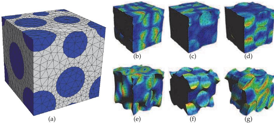
Fig. 5. Unstructured and non-periodic RUC finite element mesh (microscale). Characteristic displacements for the 30% reinforcement RUC: normal eigenshapes (a)  $\chi_{11}$ , (b)  $\chi_{22}$ , (c)  $\chi_{33}$  and shear eigenshapes (d)  $\chi_{12}$ , (e)  $\chi_{23}$ , (f)  $\chi_{13}$  (Oliveira et al., 2009).
