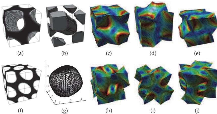
Fig. 11. Microscale topology optimisation, using the inverse homogenisation, for a 3-D RUC ( $\varepsilon=\{0;0;0;1;1;1\}$ ): (a) stiff and (b) soft material distributions, (f) periodicity illustration, (g) anisotropy plot, and (c-e,h-j)  $\chi_{11}$ ,  $\chi_{22}$ ,  $\chi_{33}$ ,  $\chi_{12}$ ,  $\chi_{23}$  and  $\chi_{13}$  characteristic displacement modes.
