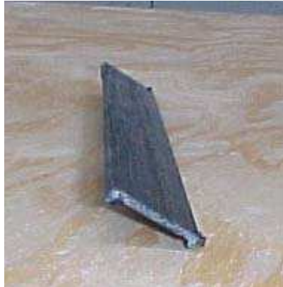
Fig. 19. U-Shape GF/PP pultruded profile made from towpregs
