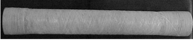
Fig. 18. Filament wound GF/PVC pipe
