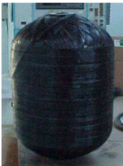
Fig. 17. Filament wound GF/PP pressure vessel processed from towpregs
