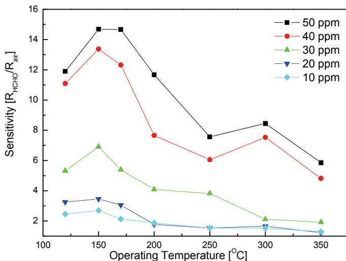
Fig. 8. HCHO Gas-sensing properties of  $\text{La}_{0.8}\text{Sr}_{0.2}\text{FeO}_3$  [17].
