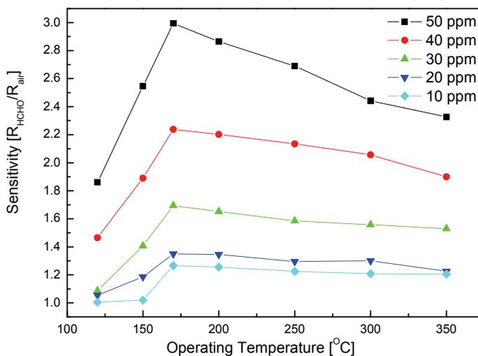
Fig. 9. HCHO Gas-sensing properties of  $\text{La}_{0.5}\text{Sr}_{0.5}\text{FeO}_3$  [17].
