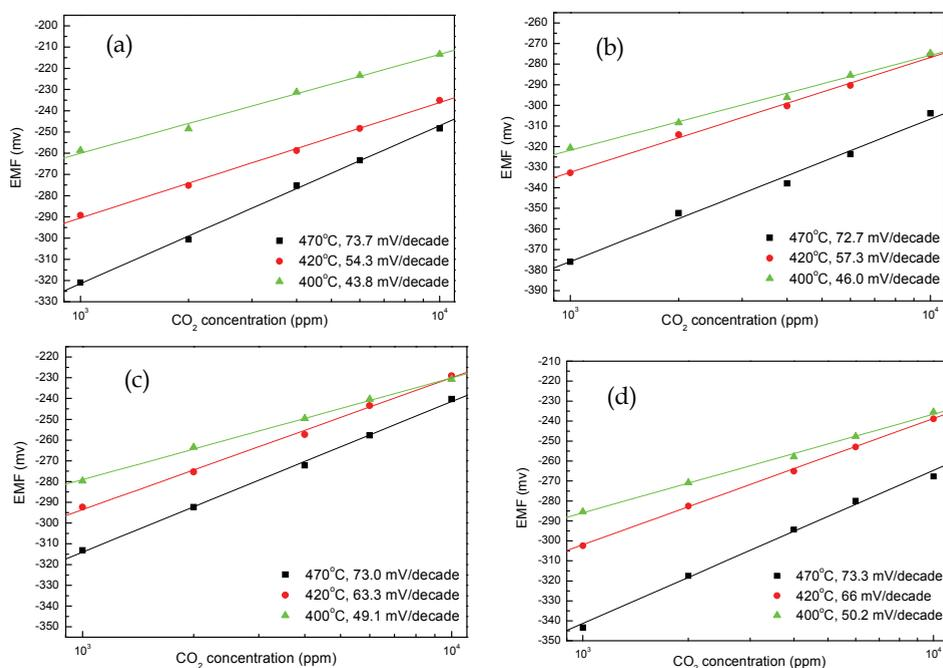
Fig. 6. CO<sub>2</sub> concentration vs. EMF for the CO<sub>2</sub> gas sensors attached with (a)  $\text{Na}_2\text{CO}_3\text{-CaCO}_3 = 1:0$ , (b)  $\text{Na}_2\text{CO}_3\text{-CaCO}_3 = 1:0.5$ , (c)  $\text{Na}_2\text{CO}_3\text{-CaCO}_3 = 1:1.5$ , and (d)  $\text{Na}_2\text{CO}_3\text{-CaCO}_3 = 1:2$  [18].
