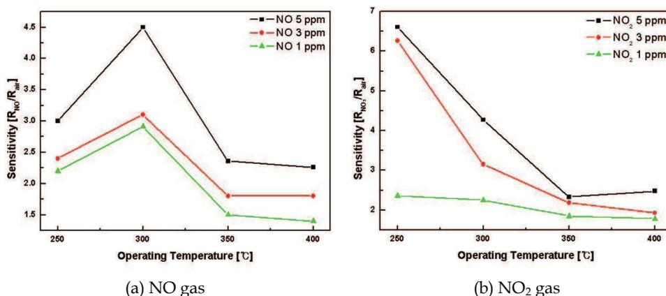
Fig. 3.  $\text{NO}_x$  Gas-sensing properties of  $\text{WO}_3$  [19].
