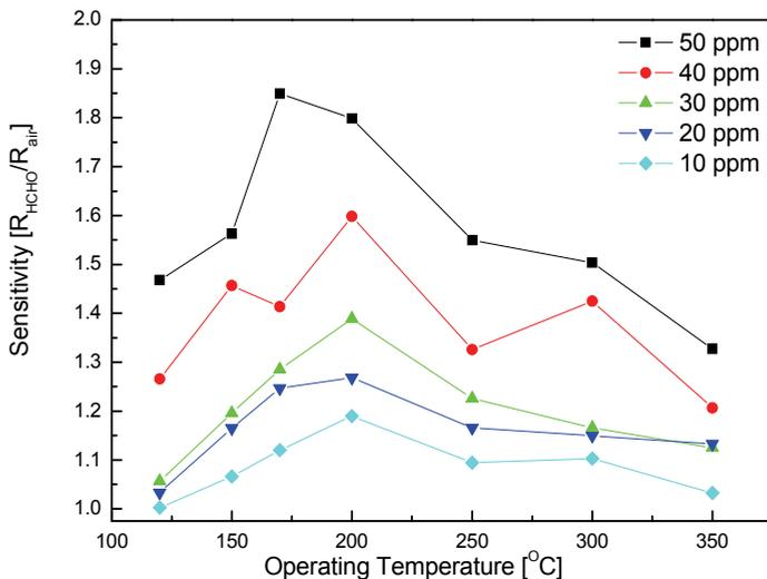
Fig. 7. HCHO Gas-sensing properties of  $\text{LaFeO}_3$  [17].
