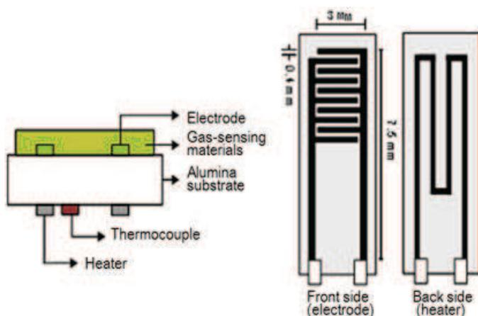
Fig. 2. Schematic diagrams of the gas sensor [19].
