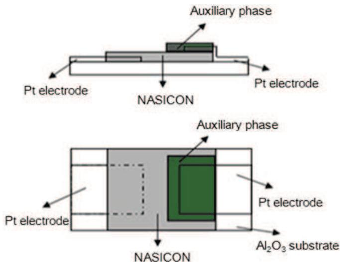
Fig. 5. Schematic diagrams of the CO<sub>2</sub> gas sensor [18].
