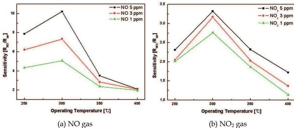
Fig. 4. NO<sub>x</sub> Gas-sensing properties of In<sub>2</sub>O<sub>3</sub> [19].
