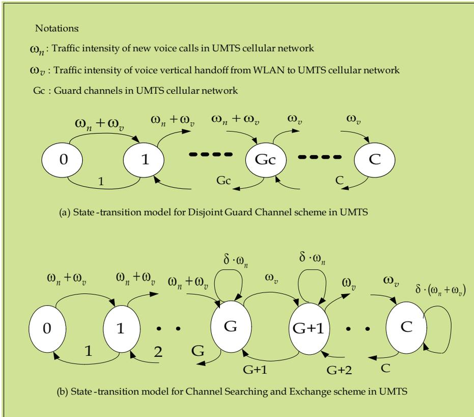
Fig. 9. State-transition diagram for DGC and CSR algorithms
