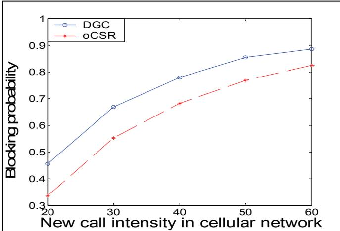
Fig. 14. Blocking probability with optimal CSR and DGC
