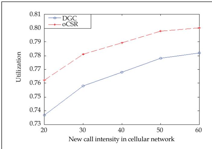
Fig. 13. Utilization with new call intensity in UMTS
