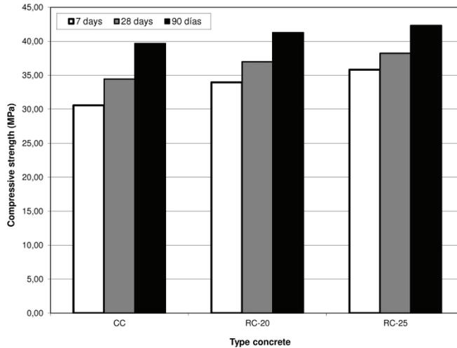
Fig. 2. Compressive strength of the concretes
