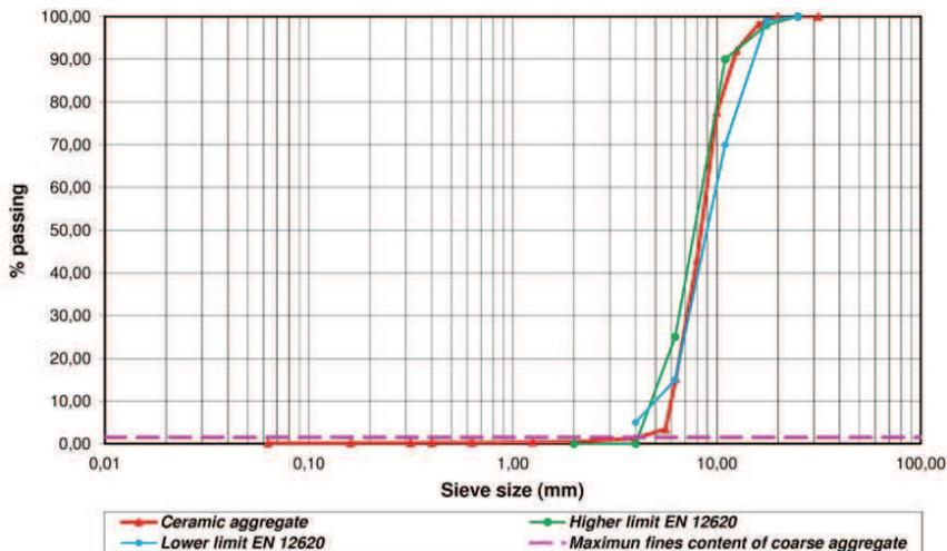
Fig. 1. Particle size grading of ceramic aggregate
