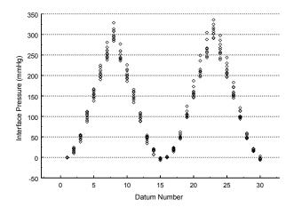
Fig. 7. Measured interface pressure data from the upper and lower arms (second inflate/deflate cycle) of 11 subjects. Inflate-deflate sequence, 0, 20, 50, 100 ...300, 250, ...50, 20,0 mmHg.
