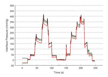
Fig. 11. Concurrent interface pressure for a CAT on the upper leg with the BIPT three sensor array placed longitudinally under the CAT. First cycle - outer leg position; second cycle - inner leg position.
