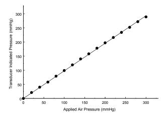
Fig. 5. BIPT calibration curve using air applied pressure (inflate-deflate cycle).
