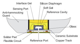
Fig. 3. Schematic representation of a gel modified MEMS pressure sensor with conformable anti-hammocking guard.
