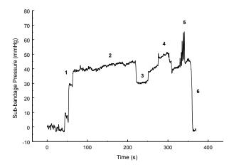
Fig. 13. Interface pressure measured with BIPT located above the medial malleolus under a Smith & Nephew ProGuide bandage: 1 Bandage Application, 2 Sitting with foot on floor, 3 Foot elevated, 4 Standing, 5 Flexing calf muscle, 6 Bandage removal.
