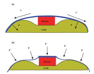
Fig. 1. Deformation of interface region due to intrusive rigid sensor. The 'Hammocking' effect for (a) Tension devices such as bandages and combat application tourniquets (CATs), (b) Pneumatic tourniquet type devices.
