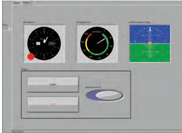
Fig. 14. The LabVIEW front panel of host PC (aircraft instruments)
