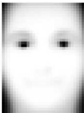
Fig. 10. Mixture coefficients of the model for face image patches. Bright pixels indicate a high probability for skin, dark pixels indicate a low probability for skin (Hoffmann et al. (2009)).
