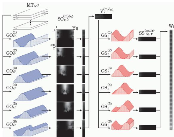
Fig. 3. Structure of the double spreading layers.
