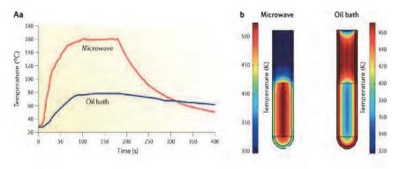
Fig. 4. Temperature profiles for ethanol under microwave radiation and open vessel oil bath condition and temperature gradient 1 min. after heating (Kappe and Dallinger 2006).
