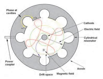
Fig. 1. (b) Construction and working of Magnetron
