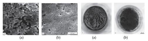
Fig. 3. Morphology with SEM micrograph of the combustion process (a) hot plate (b) microwave radiation (Park et al. 1998)
