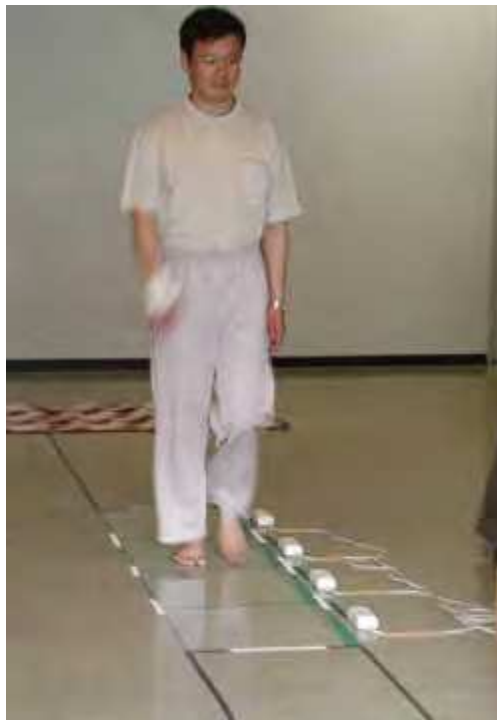
Figure 3. Pressure Distribution Measurement of Stance Foot
