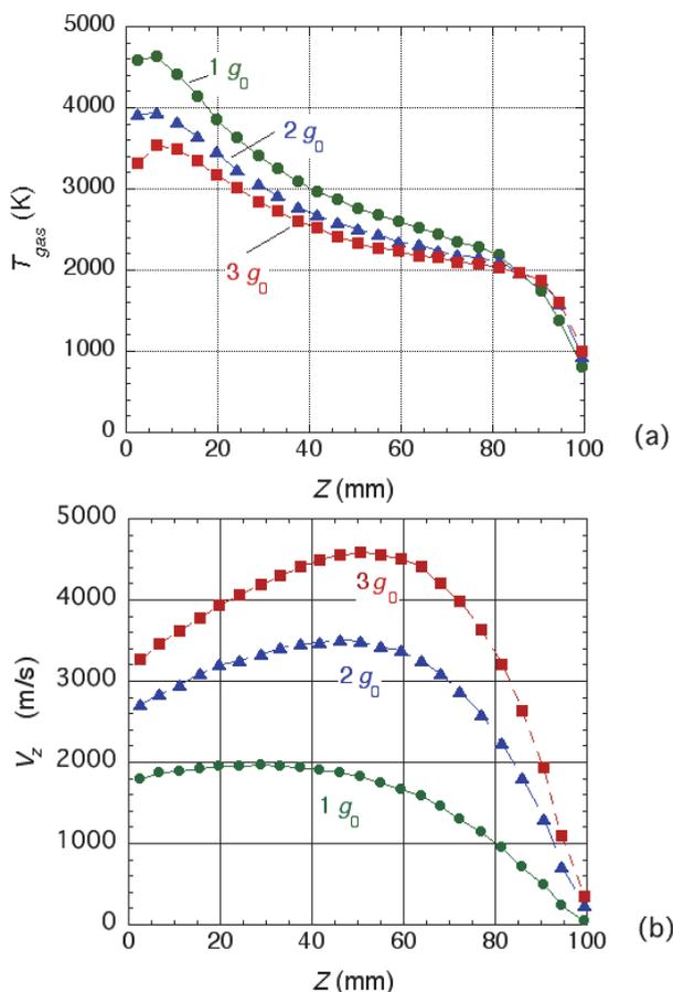
Fig. 4. (a) Vertical ( $z$ ) direction distributions of gas temperatures for gravitational strengths of  $1.0 g_0$ ,  $2.0 g_0$  and  $3.0 g_0$ , where the centre of the arc flame is set to  $z=0$  cm,  $r=1.1$  cm,  $p(\text{He})=50$  kPa and  $P_{IN}=1.0$  kW. (b) vertical direction distributions of gas velocity  $V_z$  for the three gravitational strengths.
