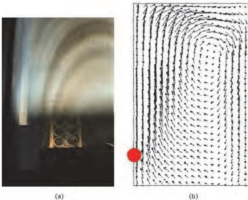
Fig. 13. (a) Mie scattering image of the carbon-cluster flow from the plasma region under  $3 g_0$  (side view).  $p(\text{He})= 50\text{kPa}$ ,  $I_d= 40 \text{ A}$ ,  $t= 4.0 \text{ min}$ . (b) Corresponding calculation of the gas velocity by the SMAC method.
