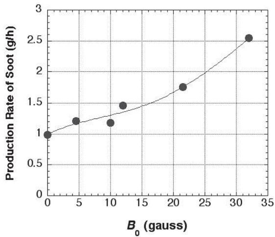
Fig. 19. Production rate of soot including SWNTs vs applied magnetic field.
