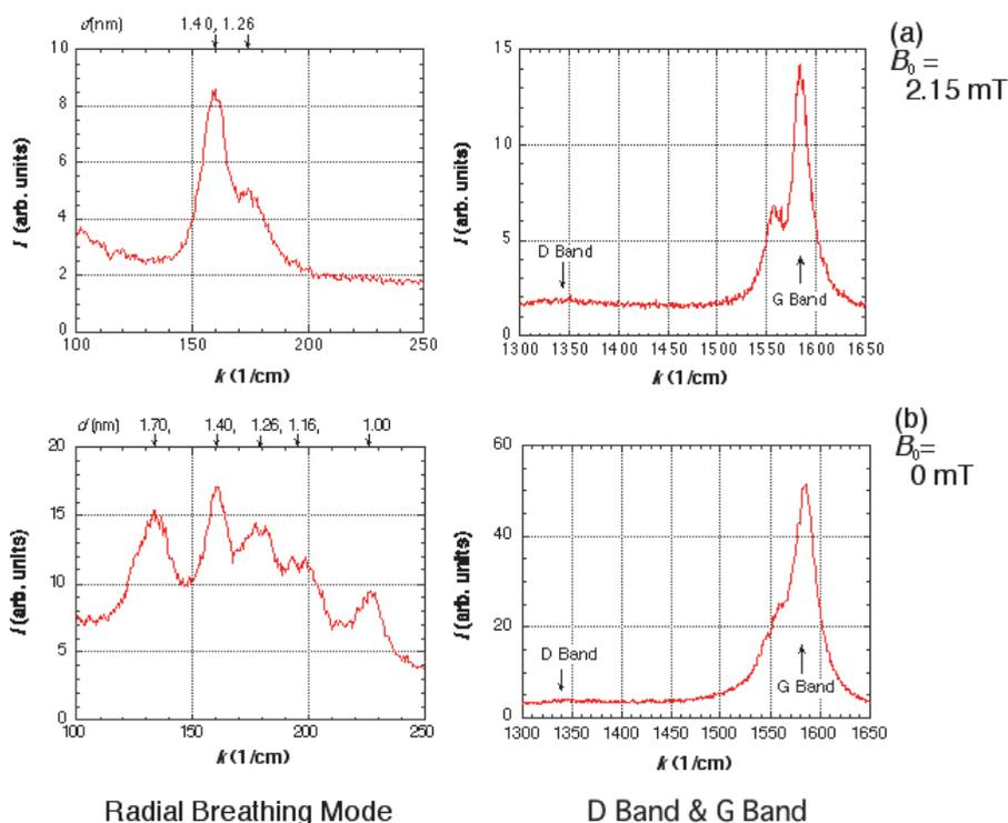
Fig. 20. Raman spectra of the soot including SWNTs under the two magnetic fields.  $p(\text{He})=60$  kPa and  $I_d=50$  A. From the RBMs in the left graphs, the diameter of SWNTs,  $d$ , can be estimated and is written on the top of the figure. In the right graphs, the peaks of the G-band and D-band of carbon are shown.
