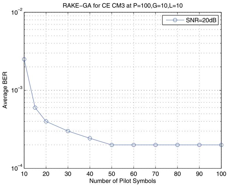
Fig. 5. Impact of Pilot size on RAKE-GA
