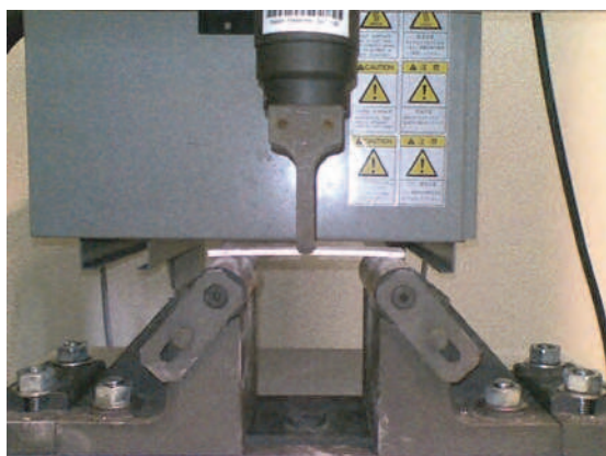
Fig. 10. Three point bending test setup
