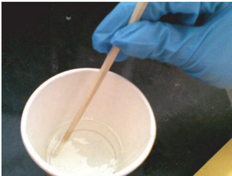
Fig. 3. Mixing of epoxy resin and hardener
