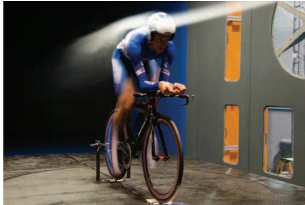
Fig. 6. Cyclist pedaling in the wind tunnel
