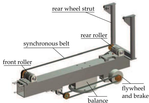
Fig. 7. The test rig for the cyclist
