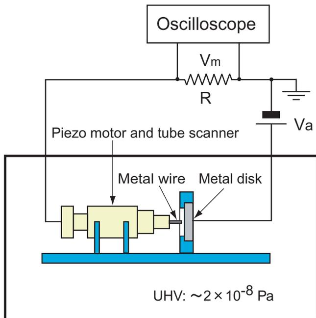
Fig. 3. An apparatus for fabricating wire-disk-type break junctions.
