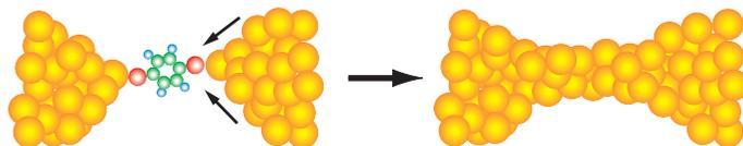
Fig. 17. Possible breakdown or collapse of electrodes at the high bias instability.
