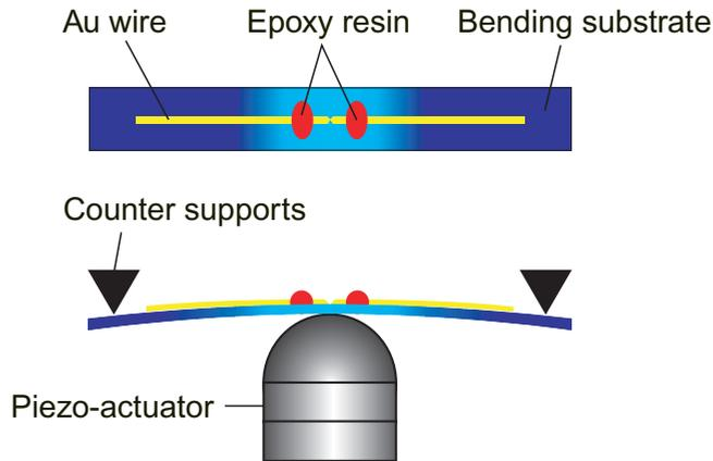
Fig. 4. Schematic of MCBJ (mechanically controllable break junction).
