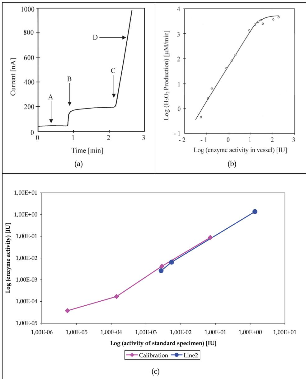
Fig. 12. a) Schematic view of enzyme activity measurement; A) addition of glucose concentration in vessel  $c_{vessel} = 500 \text{ mM}$ ; B) addition of  $H_2O_2$  for calibration  $c_{vessel} = 20.2 \text{ }\mu\text{M}$ ; C) injection of GOx solution of unknown activity; D)  $H_2O_2$  production ( $478 \text{ }\mu\text{M}/\text{min}$ ). b) Calibration curve for enzyme activity measurement using MFS (Krejci et al., 2008). c) Calibration curve for enzyme activity measurement using RDE.
