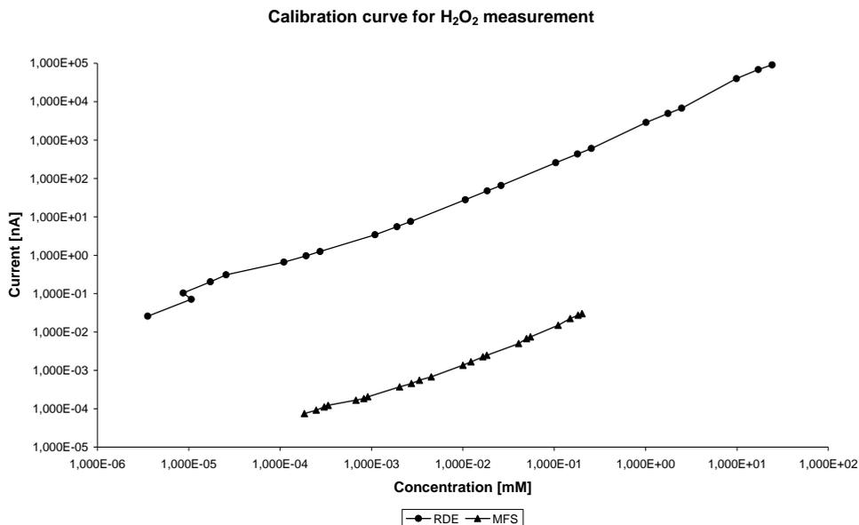
Fig. 9. Calibration curve for H<sub>2</sub>O<sub>2</sub> measurement (Krejci et al., 2008).
