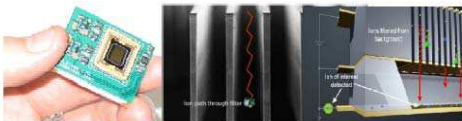
Fig. 4. FAIMS principle and chip of Owlstone Company
