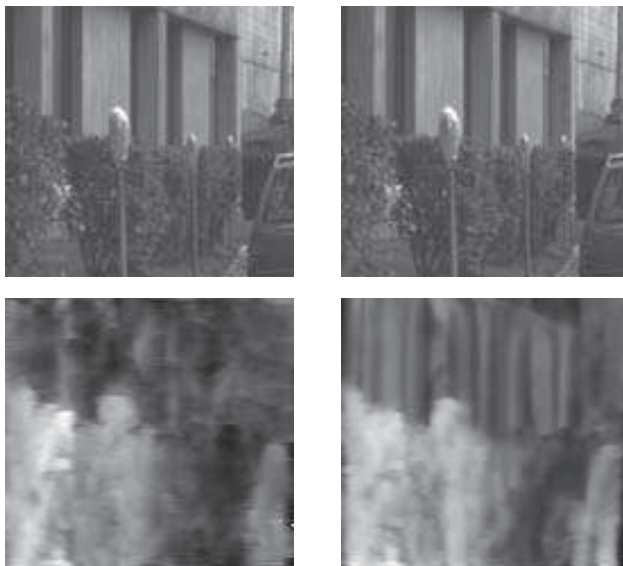
Fig. 6. Top: Meter stereo pair. Bottom: Disparity maps obtained through the whitened Green's function approach (left) and through the original approach of (Torreão, 2007) (right).
