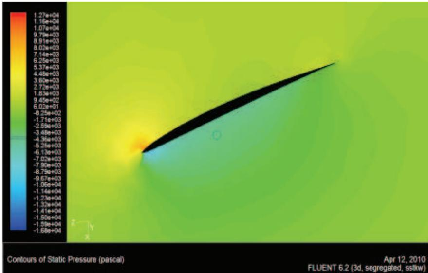
Fig. 13. Pressure contour surrounding the blade at 0.8 adv
