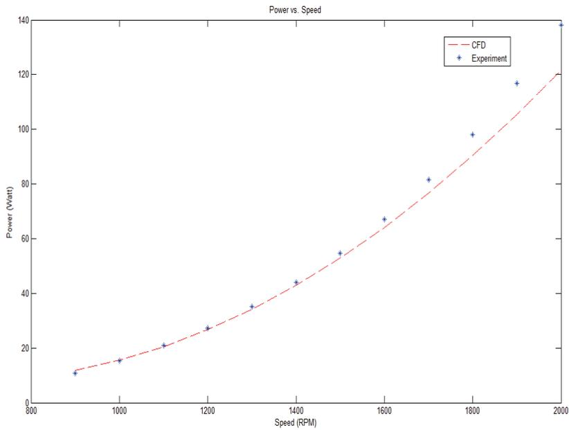
Fig. 6. Plot of power input against propeller speed
