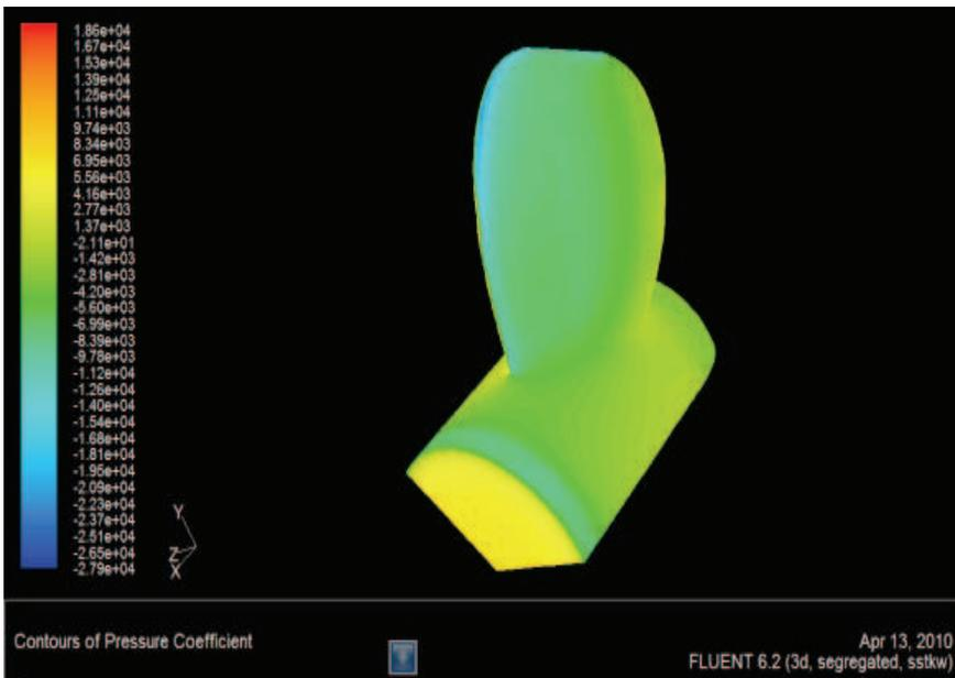
Fig. 15. Pressure coefficients at the front surface
