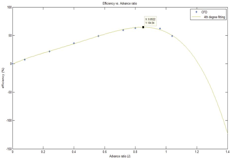
Fig. 9. Plot of efficiency vs. advance ratio
