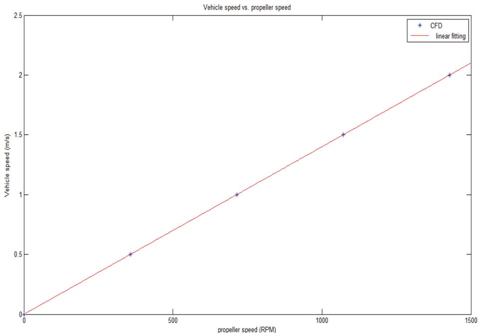
Fig. 16. Relationship between vehicle speed and propeller speed
