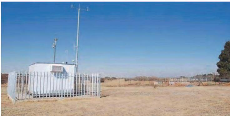
Fig. 6. Measuring station for taking particulate matter measurements
