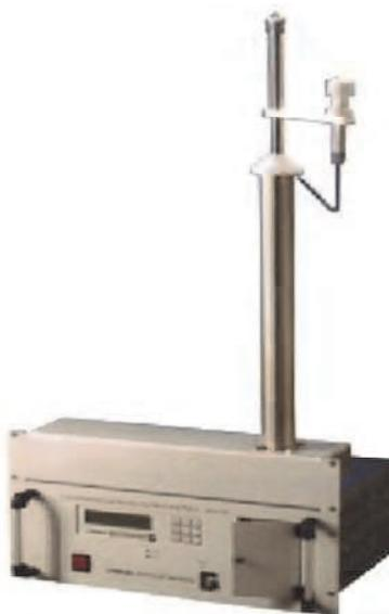
Fig. 7. Measuring equipment for taking particulate matter measurements
