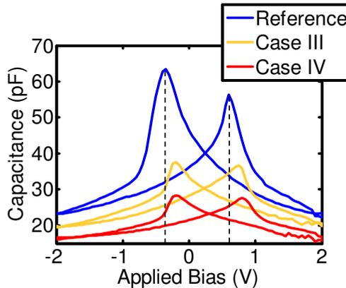
Fig. 11. Effect of the O<sub>2</sub> plasma treatments on C–V hysteresis loop curve. The built-in electric field increases after each treatment, which is indicative of Pb oxidation or O vacancy filling. The O<sub>2</sub> flow rate and pressure were varied from 100 sccm and 0.5 Torr (case III) to 500 sccm and 5 Torr, respectively (Tayebi et al., submitted).
