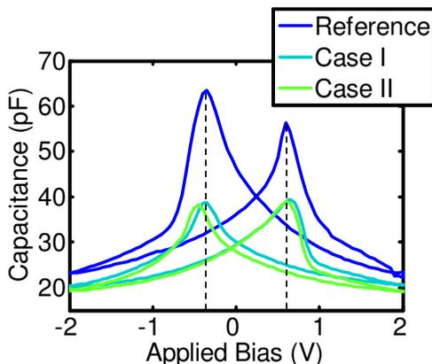
Fig. 10. Effect of the  $H_2$  plasma treatments on the variation of capacitance as a function of applied bias. The built-in electric field decreases after each treatment, which is indicative of Pb reduction or O vacancy formation. The pressure was varied from 0.5 (case I) to 1 Torr (case II), while the gas flow rate of He with 4%  $H_2$  was maintained at 1000 sccm (Tayebi et al., submitted).
