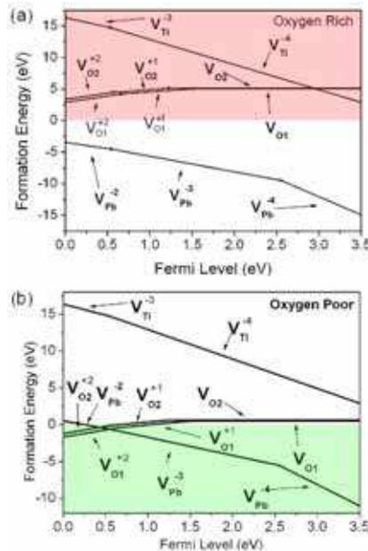
Fig. 13. Previously published *ab-initio* calculations of defect formation energy for vacancies as a function of the Fermi level in oxygen-rich (a) and oxygen-poor (b) conditions (Zhang et al., 2006). Only the vacancies among the lowest formation energies are shown.
