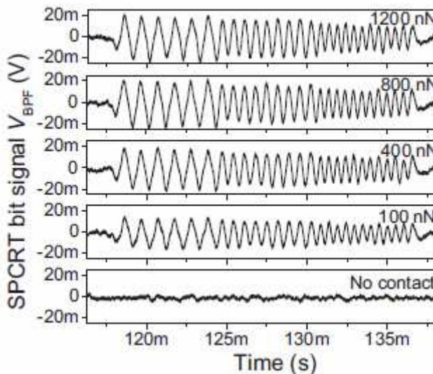
Fig. 17. Bit signal traces in time domain of the three different wavelengths (1.6, 1.2, and 0.8  $\mu\text{m}$ ), alternating polarizations at various applied forces. The scanning speed was maintained at 1.6 mm/s (Kim et al., 2009).
