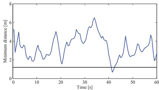
Fig. 14. The figure shows the closest distance of any person for one randomly chosen simulation. The horizontal black line, is at  $1.2m$  distance, which corresponds to the transition between the social zone and the personal zone, which the robot should try to stay out of.
