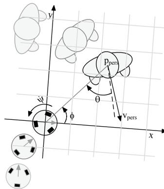
Fig. 2. The state variables  $p_{pers}$  and  $v_{pers}$  hold the position and velocity of the person in the robot's coordinate frame.  $\theta$  is the orientation of the person and  $\psi$  is the rotational velocity of the robot.
