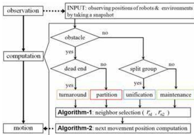
Fig. 5. Adaptive navigation algorithm flowchart
