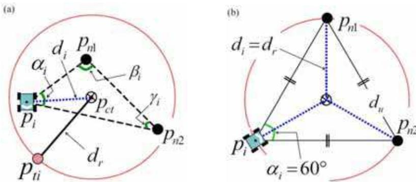
(a) control parameters range  $d_i$  and bearing  $\alpha_i$       (b) desired equilateral triangle  $\mathbb{E}_i$
